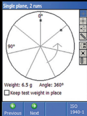
Dynamic balancing in single plane according to ISO 1940-1
