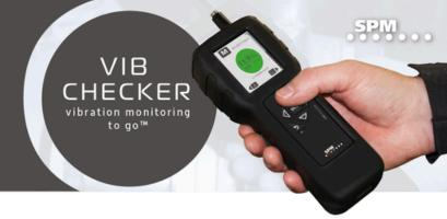
VibChecker is a compact-sized instrument for vibration measurement in the 10-1000 Hz frequency range. Measurement results are immediately and automatically evaluated against ISO standards with a clear, intuitive indication of vibration severity. Time signals and realtime FFT spectrums enable easy pattern recognition. Measurement results can be stored for trending of vibration levels and follow-up.
